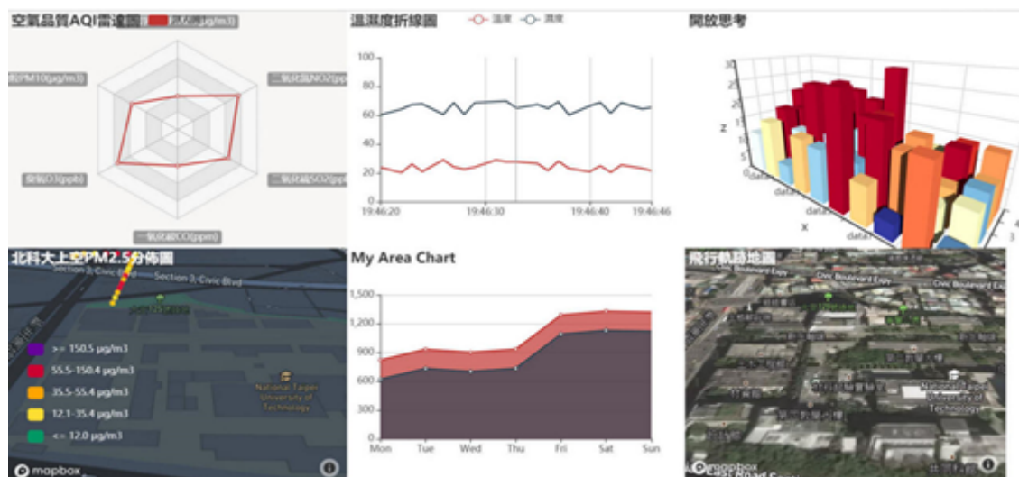
Fig. 1. Information Visualization Module Dashboard (From Left to Right, From Top to Bottom, Air Quality (AQI) Radar Chart, Temperature, and Humidity Line Chart, 3D Histogram, NTUT PM2.5 Distribution Chart, My Area Chart, UVA Flight Path Diagram)
