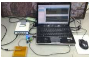
Fig. 3. Setup of FEPL tester using NI USB 4431 for SPL measurement
