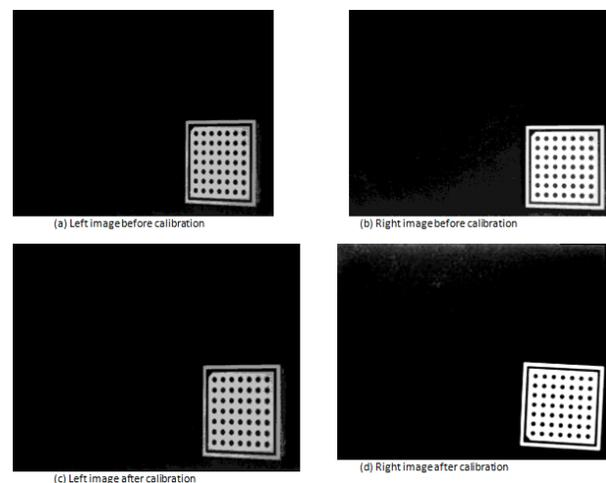
Fig. 5. The plate images were taken before and after camera calibration
