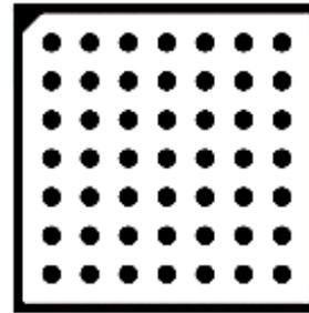
Fig. 3. A calibration plate
