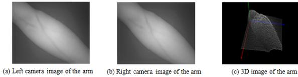
Fig. 6. Binocular stereo vision of an arm
