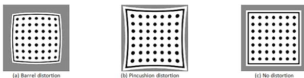
Fig. 2. Barrel, pincushion and no distortion
