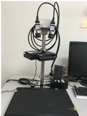
Fig. 1. A binocular stereo vision system
